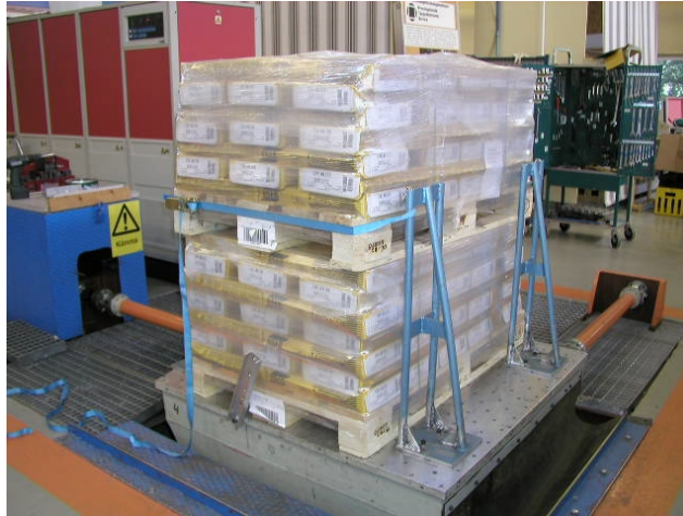
Figure 9. Test setup on vibration table, a stack of two pallets.
