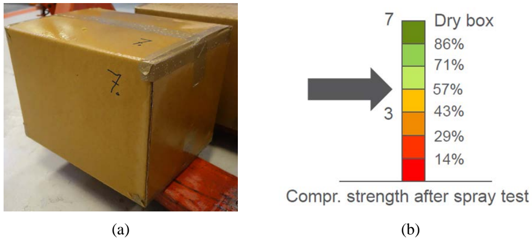
Figure 8. Wetting resistance of corrugated board: (a) Example of spray tested box; (b) Resulting BCT value after spray test in comparison with BCT value on laboratory conditioned boxes (denoted “dry” in the study).
