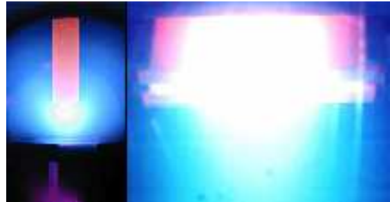
Fig. 1 Images of the hollow cathode plasma generated by the radio frequency power in cylindrical Cr cathode (left) and linear slit cathode (right). The working gas used in both systems was nitrogen, the gas pressure was 0.25 Torr. Cylindrical cathodes can be used for inside treatments.
