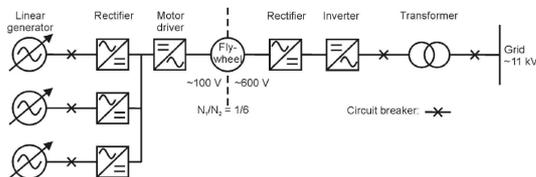
Figure 12 – Circuit diagram of the proposed system applied on linear wave energy converters
