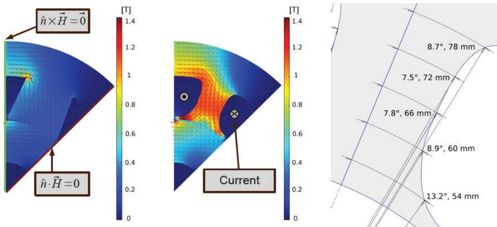
Figure 11 – From left to right; the original geometry based on a constant average area of the magnetic flux. The optimized geometry and a sketch of the geometry with the optimization variables.
