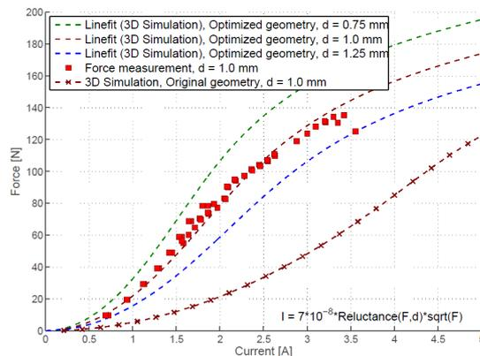
Figure 10 – Measured force from the magnetic bearing as a function of current and comparison with simulations. Nominal value of the air gap,  $d$ , is 1.0 mm.
