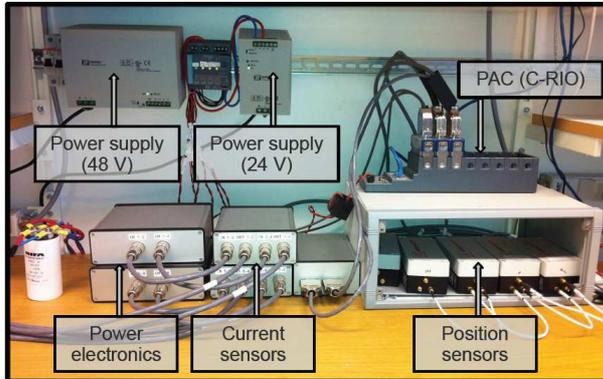
Figure 9 – Schematics of the magnetic bearing control and the lay out in the lab.
