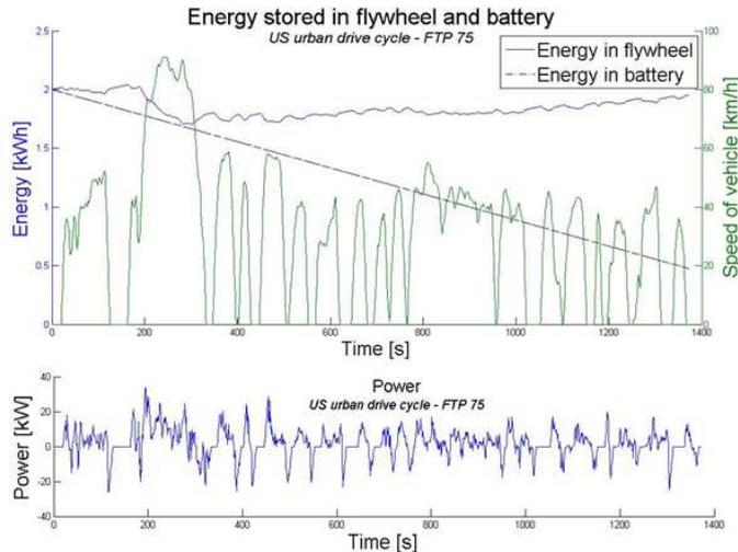
Figure 11 – Drive cycle for passenger car (FTP 75), showing a steady supply of energy from the battery can be complemented by a flywheel that handle power peaks. The average power is only 4 kW, while the peak power is up to 36 kW.
