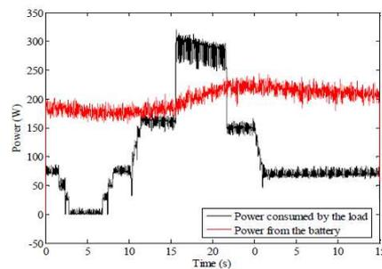
Figure 4 – Power consumed by the load and the battery from the battery during an experimental test.
