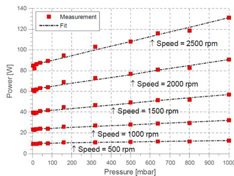
Figure 2 – We studied the air friction loss at different rotational speed and air pressure. Results have been published in [5].
