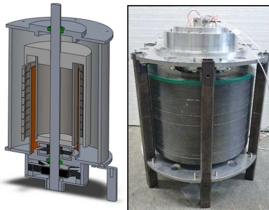
Figure 8 - Cut away drawing representation of the flywheel machine and current construction status.
