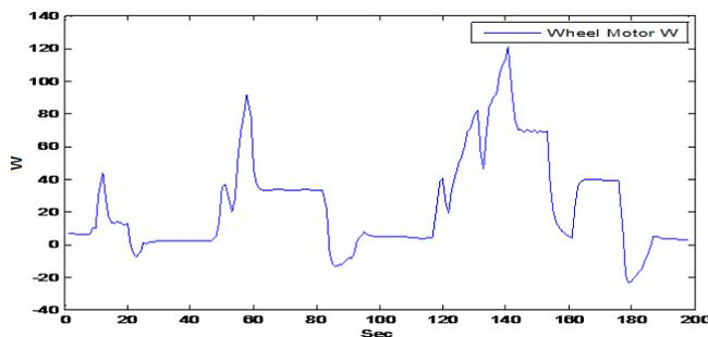
Figure 8 – Measured electric power in the input terminals of the traction motor.
