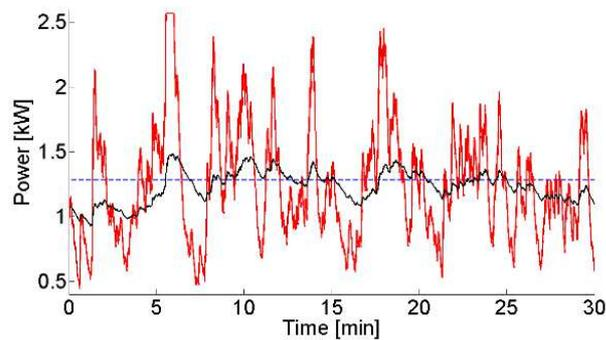
Figure 13 – power out from the flywheel with flywheel energy storage capacities of 50 kJ (red) and 500 kJ (black) respectively.
