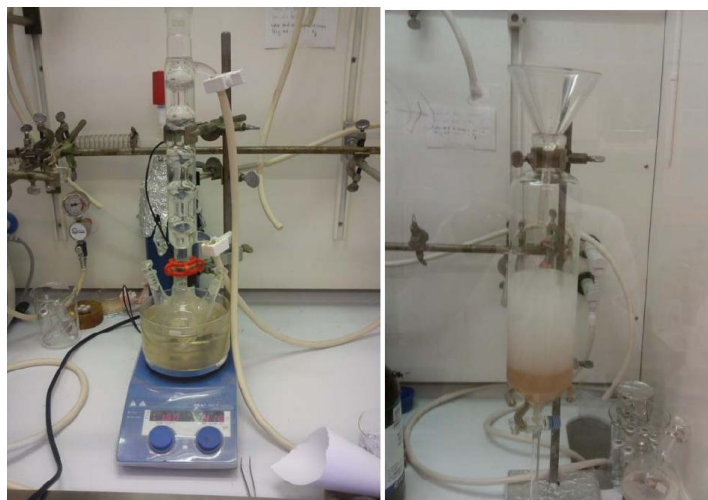
Figure 1. a) liquefaction of waste paper, b) purification of plasticizer.
