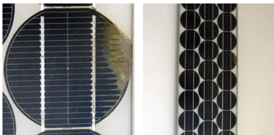
Figure 14: To the left: The cell with a clearly visible degradation. To the right: The module where the degraded cell is fitted
