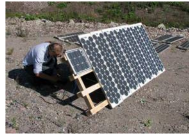
Figure 4: The arrangement for measuring the Bullerö modules.
