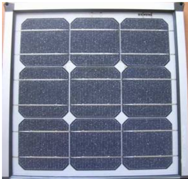
Figure 3: The Siemens reference cell that was used for measuring irradiance and cell temperature.
