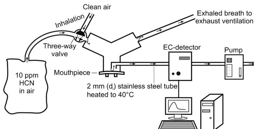
**Fig. 1.** A schematic description of the experiment setup where the volunteer is exposed to 10 ppm HCN gas for 1 min. Thereafter, the inhalation is switched to clean air. Breath is continuously pumped from the mouth orifice via a heated stainless tube to the electrochemical detector. Thus, the sample consists of a mixture of exhaled and inhaled breath. The results are logged to a personal computer.
